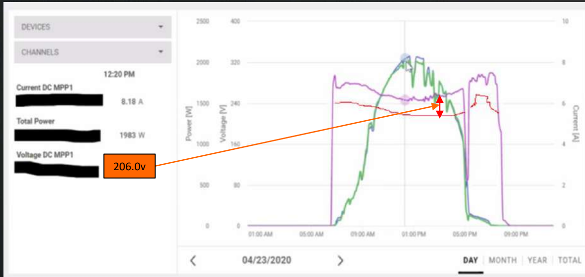
Performance: MPPT DC Voltages drop
